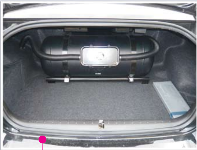
LPG鋼瓶置放後行李箱位置。 LPG steel cylinders were put in the trunk.
